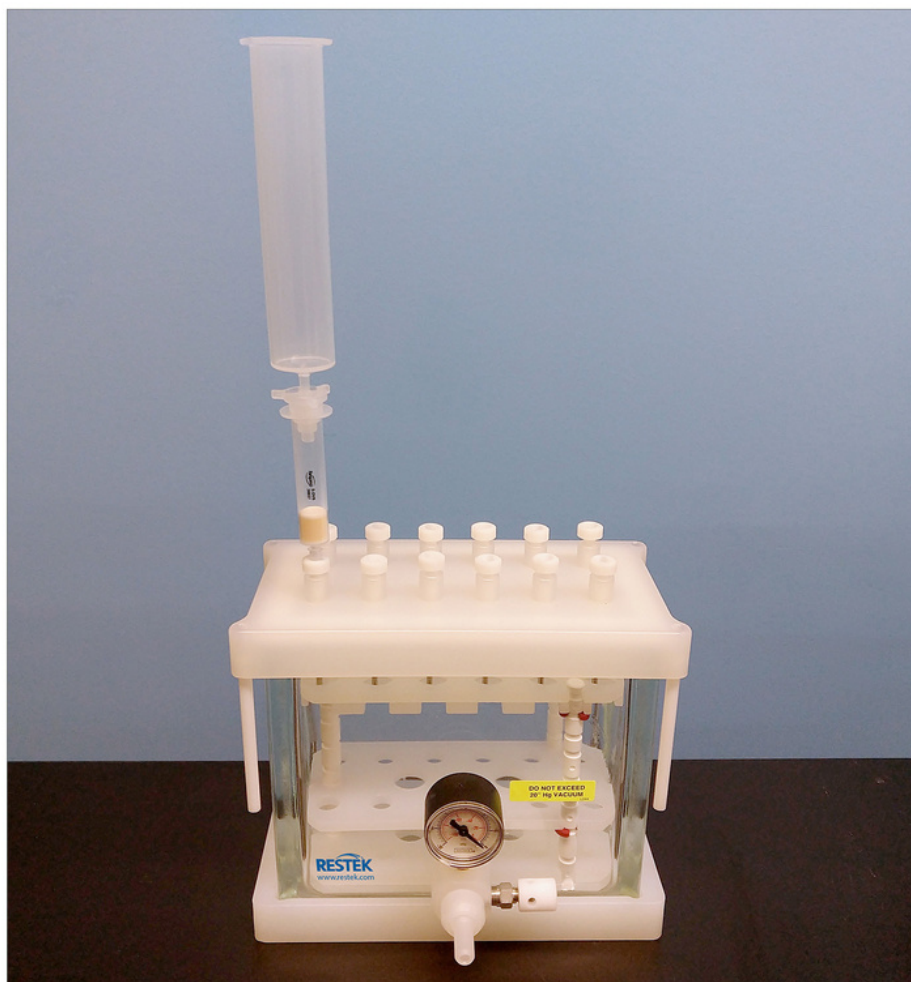
Figure 1: Sample preparation setup using sample reservoirs attached to Resprep S-DVB SPE cartridges mounted on a vacuum manifold.
